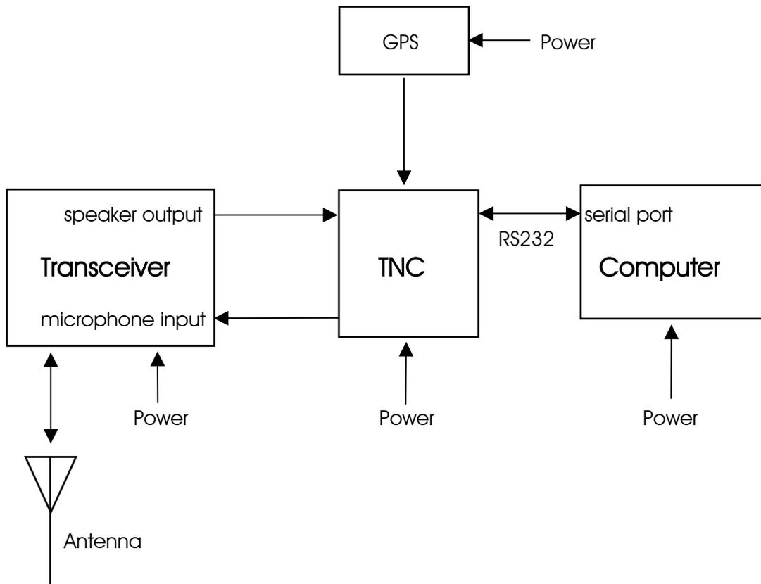
Automatic Position Reporting System (APRS) is a packet radio system used for tracking objects, people, vehicles, boats, aircraft, manned/unmanned balloons, weather systems, etc. APRS uses an Amateur Radio mode called unconnected (U) packets.
