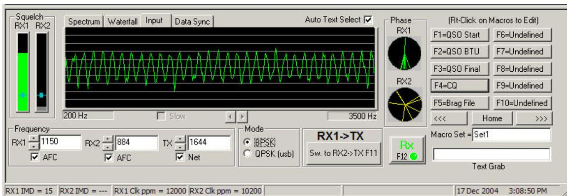
Tune the radio to a loud signal or carrier at 14,070.150 kHz. Display the soundcard's mixer program (or use the one that comes with Windows). Set the mixer's LINE IN setting to mid way. Adjust the volume control on the radio while viewing the INPUT signal display in the software program. The volume should be adjusted for a good signal level that is not too high and not too low.
