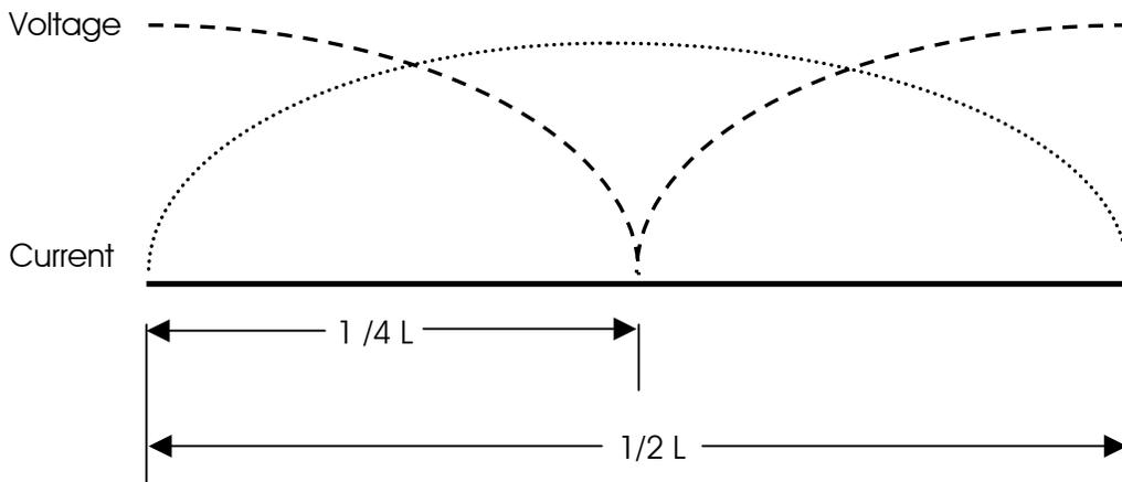
The voltage and current waves of an antenna are 90 degrees out of phase with each other.
