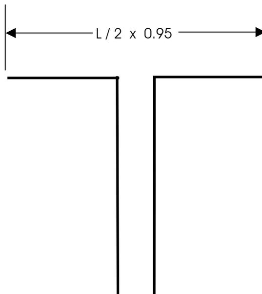
A 7 MHz. half wave dipole length =  $(c / f) \times 0.95 \times 0.5$  meters
